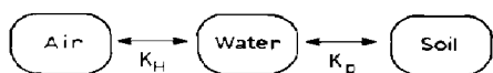
Fig.1. Three-phase system. K_p is the soil-water partition coefficient, and K_H Henry's constant.
